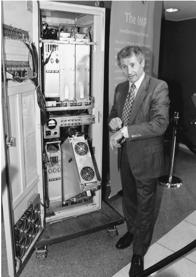
Figure 1.26 ♦ An early interface message processor (IMP) and L. Kleinrock (Mark J. Terrill, AP/Wide World Photos)
