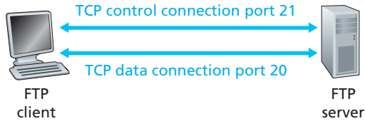
Figure 2.15 ♦ Control and data connections
