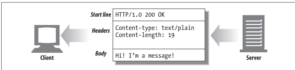
Figure 3-3. Three parts of an HTTP message
