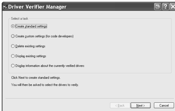
Figure 7-8 The Driver Verifier Manager in Windows XP and Windows Server 2003
