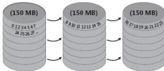
FIGURE 8-10 Logical numbering of physical sectors on a striped volume
