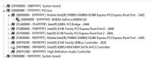
FIGURE 9-46 Hardware-reserved memory ranges on a 32-bit Windows system
