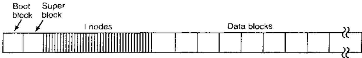
Figure 10-31. Disk layout in classical UNIX systems.
