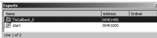
Figure 25-3: Exports window showing a TLS callback function
