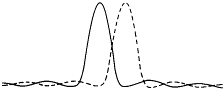
Fig. 30-6. Illustration of the Rayleigh criterion. The maximum of one pattern falls on the first minimum of the other.
